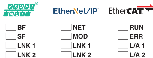
Figure 30 LED status indicators for PROFINET, EtherNet/IP™, EtherCAT®
