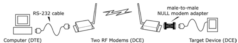
Figure B.3. Example of a Digi Radio Modem (DCE Device) connecting to another DCE device
