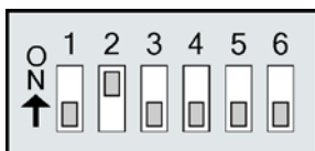
Figure 2.10. RS-485 (4-wire) and RS-422 DIP Switch Settings
