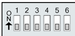
Figure 2.6. RS-485 (2-wire) Half-Duplex DIP Switch Settings
