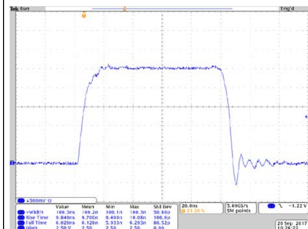
PCO-7121 (50 A, 100 ns, shorted load, inverted waveform)
