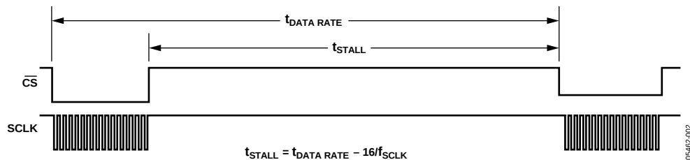
Figure 2. SPI Chip Select Timing
