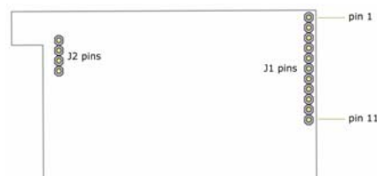
Figure 1-02. XStream OEM RF Module Pin Numbers (bottom view, pins protruding)
