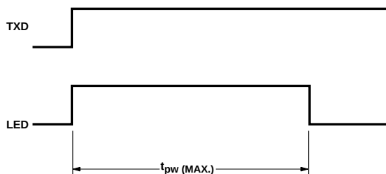
Figure 5. TXD "stuck on" protection waveform.
