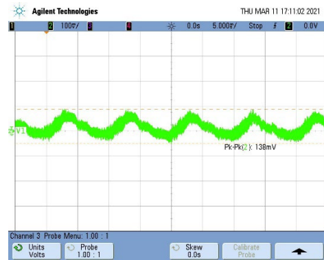
Ripple & Noise; PQU1000-54; Full Load: 264Vac Input
