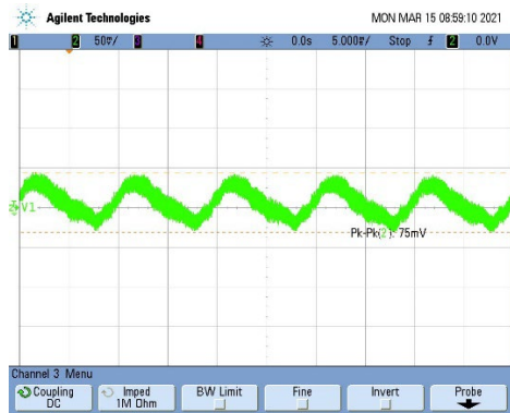
Ripple & Noise PQU1000-48; Full Load: 264Vac Input
