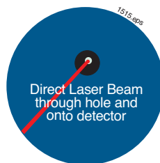
Figure 4. Close up view of the alignment laser beam to receiver aperture.
